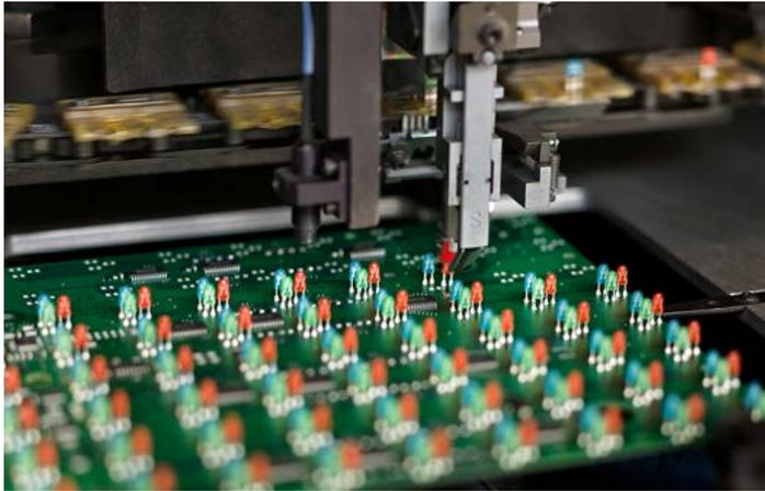
Watchfire sources the best available LEDs and components from all over the world. These through-hole LEDs are being added to a circuit board in our Danville factory.
